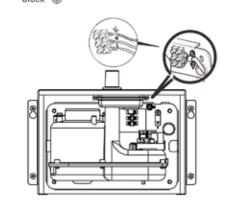
Remove end cap from blind plug. Pull wires and earthing through the flexi hose and air branch on motor. Fasten the flexi hose to the cabinet branch. Attach the opposite end of the flexi hose to branch on tap.
